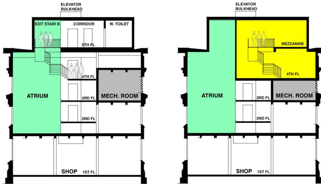
Figure 5. Schematic section through the as-built fifth-story roof-top enclosed spaces and atrium, which cannot be defined as a mezzanine (left); contrasted with a section showing a hypothetical example of a Code-compliant mezzanine within a fourth-floor room or space (right). Drawn by Jonathan Ochshorn.
